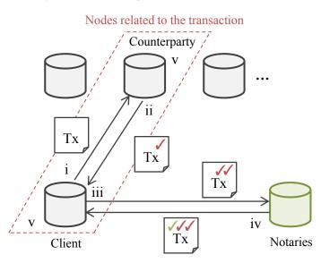
Figure 2: Execution process of transactions in Corda
