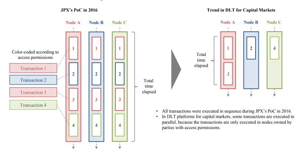
Figure 5: Parallel execution of transactions
